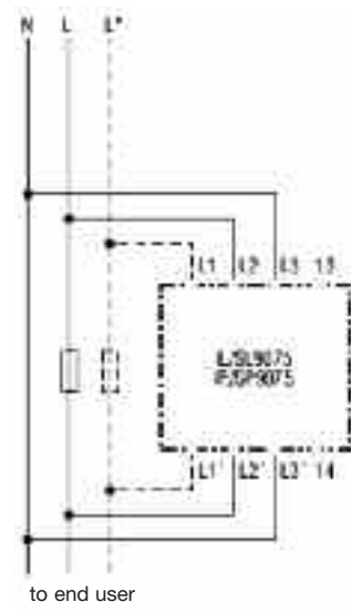
Fuse-monitoring in AC-network
